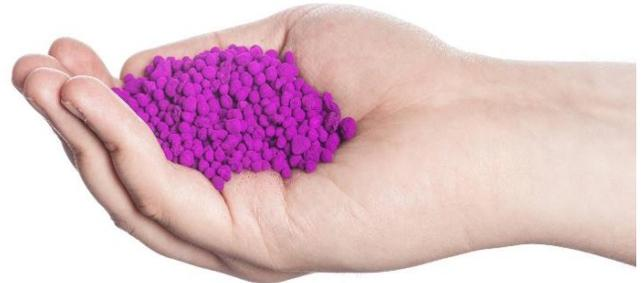
**Purafil Select Media** consists of generally spherical, porous pellets formed from a combination of activated alumina and other binders, suitably impregnated with potassium permanganate (KMnO<sub>4</sub>). The potassium permanganate is applied during pellet formation such that it is uniformly distributed throughout the pellet volume and is completely available for reaction with target gases.
